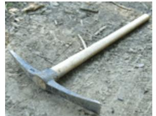
The other end is a kind of sharpened hoe blade, which can be used as a lever to shift around the broken rock. This axe end of the pickaxe can also be used to break up hard earth or cut through roots. Unlike a sledge hammer, the pickaxe blades, especially the axe end, *can* be bent if you apply enough force, so please don't.
